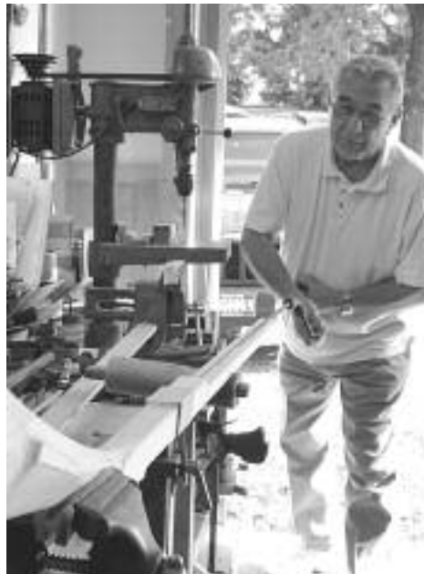
HANDLE WITH CARE: After the gun's stock is carved, a hand-crank drill bores a ramrod shaft the entire length of the barrel.
