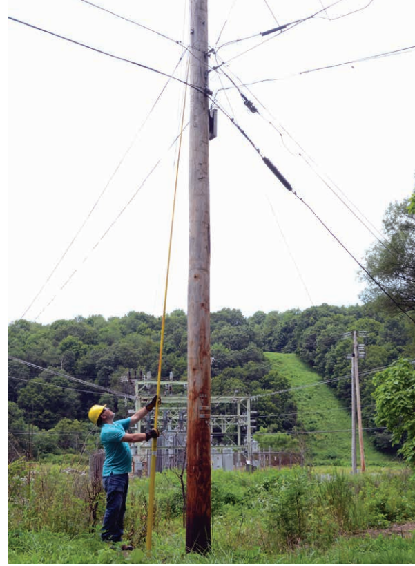
MEASURING UP: Jason Hey, a staking technician in Valley REC's Martinsburg District, checks the clearance between a telecommunications line and the co-op's electric line. The co-op's Puzzletown substation can be seen in the background.
